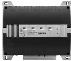
4 AC Motor Controller Wago
